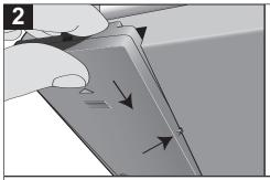
**TO INSERT:** Align the tabs from the Battery Pack into the holes on the middle of the main unit. Then, slide the Battery Pack into the main unit until it clicks into place.
